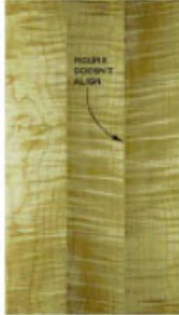
Glued up curly boards may not go well together. Curly figure is unusual because it runs at right angles to the edge of the board. It's difficult to align figured wood like this in a group of narrow boards. Instead look for wide boards
