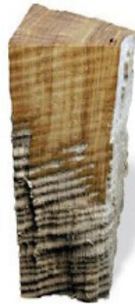
Split open a curly log and you'll find grain that bends back and forth like a wave, producing a shimmering effect like light bouncing off the ripples on a pond This chunk of white oak is spectacular-looking wood
